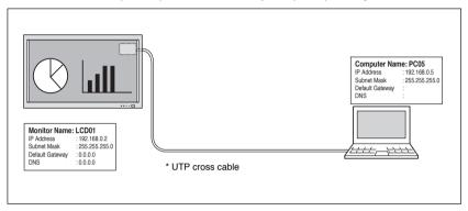
Connect the monitor (LCD01) to the control computer (PC05) via the hub.
